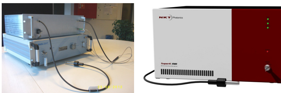
Figure 12: MINERVA supercontinuum source development. Left: the prototype mid-IR supercontinuum source at the beginning of the project. Right: The SuperK MIR product launched at the end of the project.
