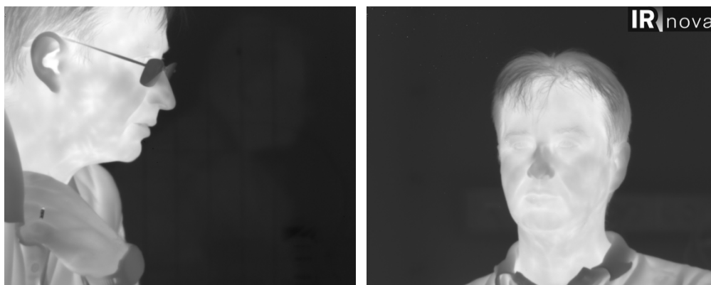
Figure 19: Images taken with a demonstration camera using new product from IRnova. The IRnova640LW is a detector with a resolution of 640×512 pixels on 15 \mu\text{m} pitch based on QWIP technology with good sensitivity in the 8-12 \mu\text{m} range. [Note the cool hair.]
