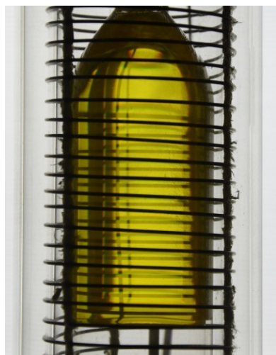
Figure 4: Calomel boule, diameter 35 mm (above)
