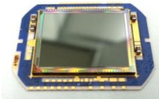
1280 × 1024 MW FPA hybridized to Xenics ROIC
