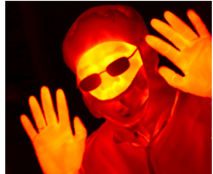
Image using a 320×256 MWIR T2SL detector taken at 110 K [Courtesy of IRnova.]
